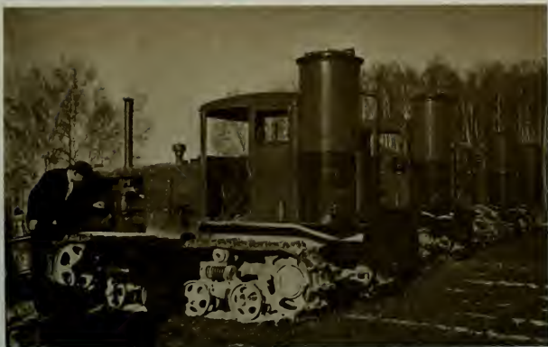
Charcoal-burning or wood-burning tractors at a Machine Tractor Station, 1939.
